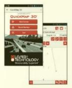
Use just a tablet app and a laser rangefinder to collect the points you need, edit errors in the field, and email the CAD-ready map.
